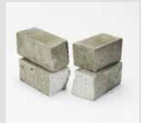
TWO SPECIMENS, THE ONE ABOVE UNTREATED, THE ONE BELOW PROTECT-TREATED,
